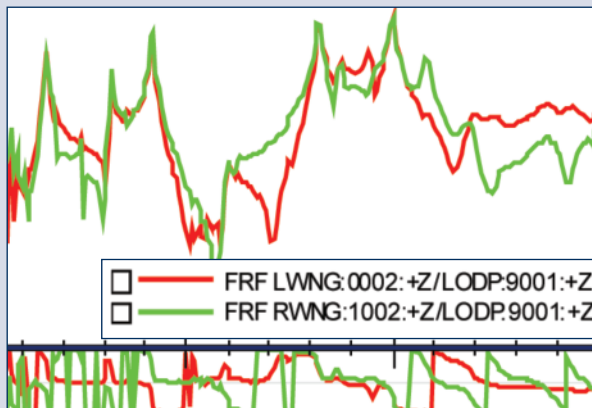
F16 wing Frequency Response Function (FRF)
