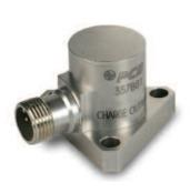
While most engine monitoring applications dictate custom designed accelerometers, some engine health monitoring requirements can be met by catalog sensors. These case isolated sensors feature differential electrical output and mount on ARINC standard PCB® also structural interfaces. supplies hard line mineral insulated cables and connectors to complement this line of catalog accelerometers. The capabilities of a few of these models are summarized below.
