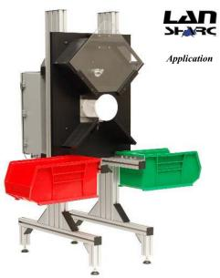
being rugged enough for the manufacturing environment. The Drop Test Fixture provides free-free testing of small parts; there is no damping of the resonant frequencies from boundary conditions such as fixtures that can decrease the resolution of the testing.
