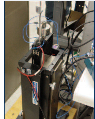
Low-frequency Accelerometer Calibrator 6" (152 mm) stroke shaker provides displacement for calibrations to 0.5 Hz
