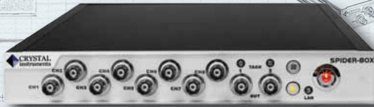
NETWORKED MODULES ACCURATE TO 50ns AT A DISTANCE OF 300 METERS
